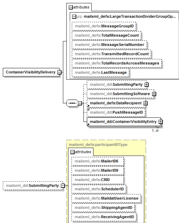
Figure 2.2: ContainerVisibilityDelivery XSD Components
