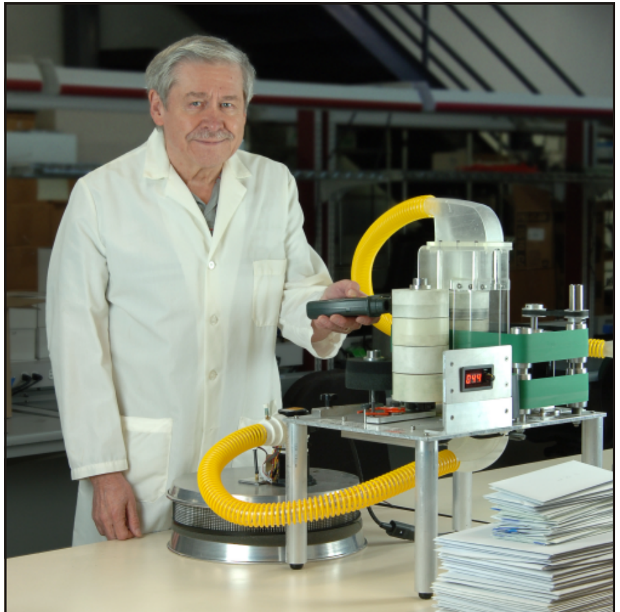
Research International CEO Elric Saaski measures RPM on a Trittek mail sorting test bed modified to support high-speed aerosol threat detection.
