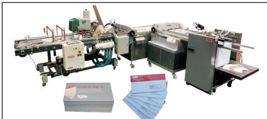
the mail finishing process. The uniqueness of this system allows the user to process multiple-up mail pieces and perform numerous functions in one pass. Direct mail pieces are edge trimmed, slit, scored, and perforated, in both directions; "T" & "L" perfs applied for tear-out reply cards or coupons, remoistenable glue is applied followed
